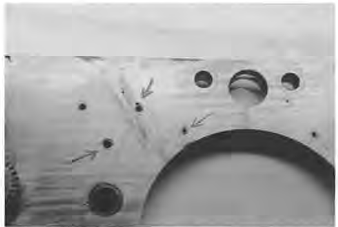
Figure 15. Extreme pivot hole wear in the train bridge. Note the two previous repairs using a prick punch in an effort to move metal into the severely worn holes and thereby trying to upright their respective train wheels. Note, also, a previously installed bushing. It showed almost no wear even after many years of service.
