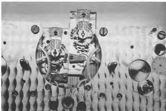
Figure 18. Installing the platform escapements by gently sliding into position.
