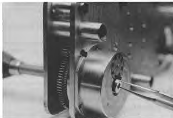
Figure 11. After putting slight pressure on the mainspring arbor in the direction of wind, the stopworks can be removed.
