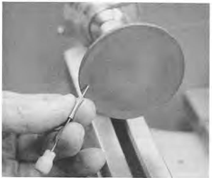
Figure 17. Grinding the center drill bit.
