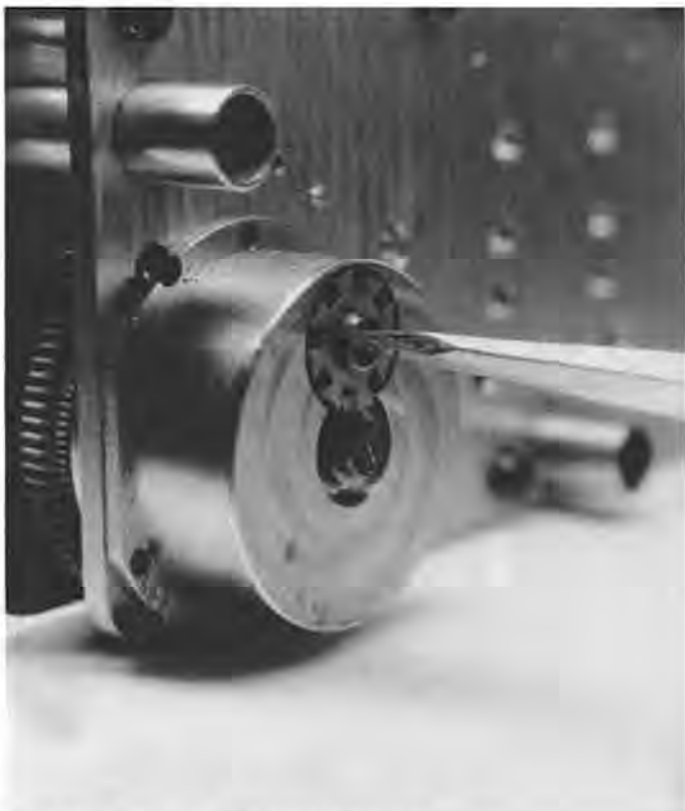
Figure 10. Removing the stopworks screws.
