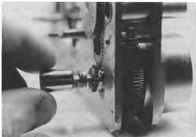
Figure 8. Removing the friction tight winding guides and winding pinion. Note the minute recording pinion and its white porcelain dial.
