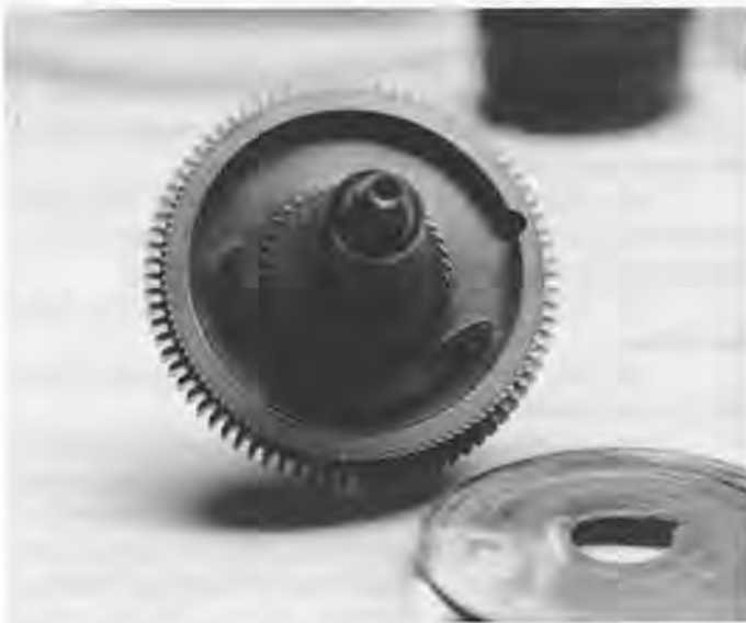
Figure 16. Main wheel winding ratchet and clock recessed on the underside of the main wheel (barrel side).
