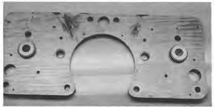
Figure 17. Idler gear on top plate connecting the main wheel with the hour wheel.
