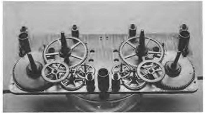
Figure 14. Both movement trains exposed.
