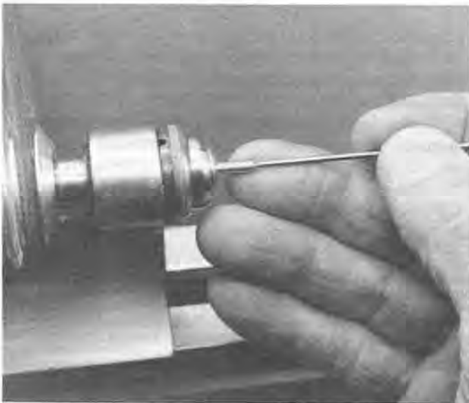
Figure 15. Test truth of running center with a very sharp scribe.
