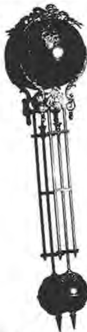
FIGURE 15. An inverted pendulum concentrates its mass in the clock movement. Adjusting the height of the ball regulates the beat.
