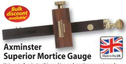
Unique to Axminster, this marking and mortice gauge is made from carefully selected rosewood and brass. Brass wear strips are inlaid into the gauge's head. Locking the head onto the stem is by means of a knurled brass thumb screw underneath which is a pressure plate to protect the stem from bruising. The lower movable pin for mortice marking is adjusted via a brass screw slide giving precise micro fine control. Maximum capacity 110mm.
