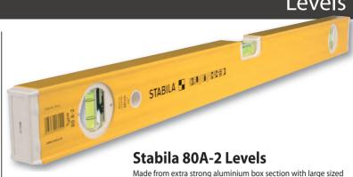
Made from extra strong aluminium box section with large sized shock absorbing end caps, one milled reference face (on models up to 2,440mm(48")), one horizontal and two plumb vials. A convenient hole is provided to hang the level when not in use.
