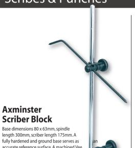
accurate reference surface. A machined Vee groove in the base allows the gauge to be used on curved surfaces. A Vee groove at the front end lets the spindle adjust to any angle above or below the base, allowing it to be used both as a height gauge and a depth gauge. Two retractable pins allow the gauge to be
