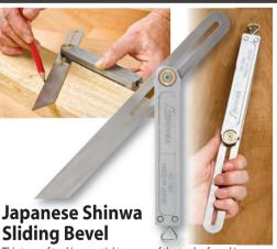
This type of tool is essential to many of the trades found in woodwork. The Shinwa sliding bevel features an anodised aluminium stock and a 1.5mm thick stainless steel blade. The best aspect is the locking mechanism located on the end of the stock so it never gets in the way. The thumb screw clamps the blade very firmly, and allows the bevel to be flipped for use on either side. The blade can be set at any angle from 0 to 180°. Use to transfer or lay out angles. Stock 150mm, blade 250mm.
