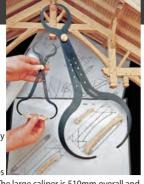
of 1:1, 1.5:1, 2:1, 3:1 and 4:1. The large caliper is 510mm overall and has the same ratios as the small plus three more: 1.25:1, 1.75:1 and 2.5:1.Both have a firm joint system where you adjust the amount of joint friction you want with the knurled brass thumbscrews The arms are anodised aluminum. These are useful for scaling up or down as well as direct measurement transfer.
