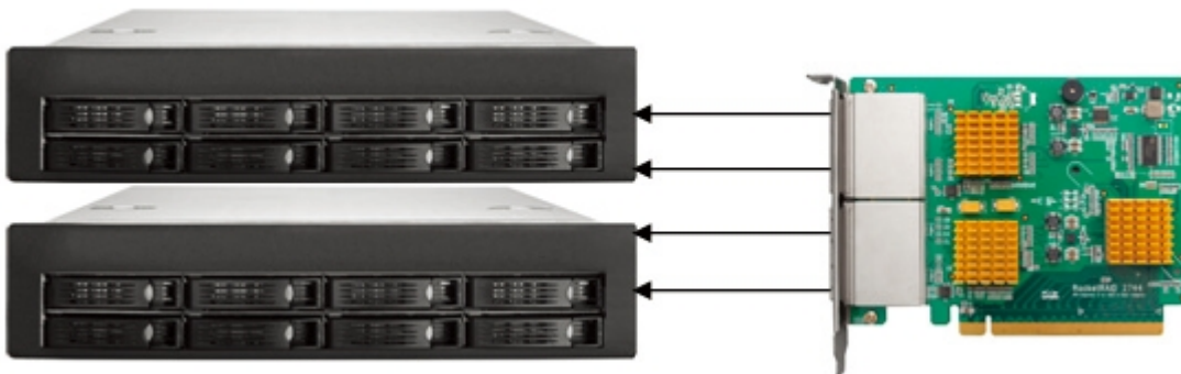
4 x SFF-8088 supports 16 HDD (Target Storage Devices)
