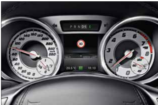
The information from Speed Limit Assist is shown both in the instrument cluster and in the COMAND Online central display.
