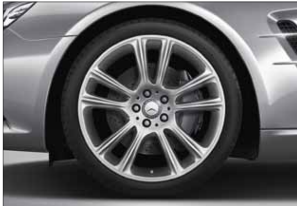
5-twin-spoke light-alloy wheels, painted vanadium silver, with 255/35 R 19 front tyres and 285/30 R 19 rear tyres (option, Code R17).
