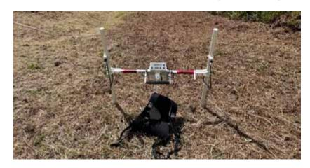
Magnetic Gradiometer. Photo credit Siobhán Ní Sheasnáin.
