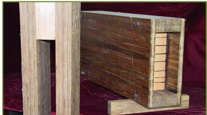
Figure 4. Moulded bamboo structural components - box-beam and splint-column made from bamboo laminated panels (fig. 2 from Wang & Guo, 2014).
