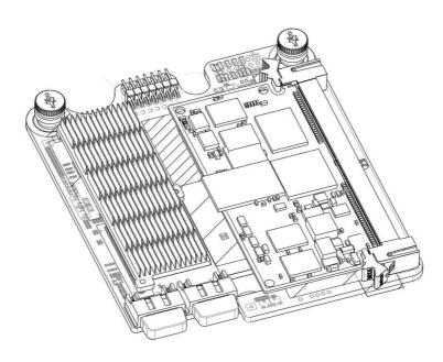
The HP Smart Array P712m mezzanine card is the preferred high value solution for 6Gb/s Shared SAS Storage for the HP ProLiant BladeSystem servers. It is one of the highest performing controllers in the SAS portfolio and provides new levels of reliability for the HP BladeSystem through its support of the latest SCSI technology and advanced RAID capabilities. Supports up to 4 P2000 Smart Arrays.
