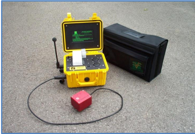
Figure 24 – Example blasting Seismograph for monitoring PPV and air-overpressure
