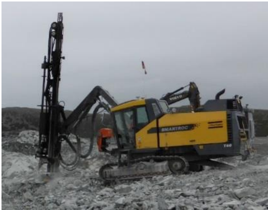
Figure 15 Example of tracked drilling rig suitable for uneven ground conditions.
