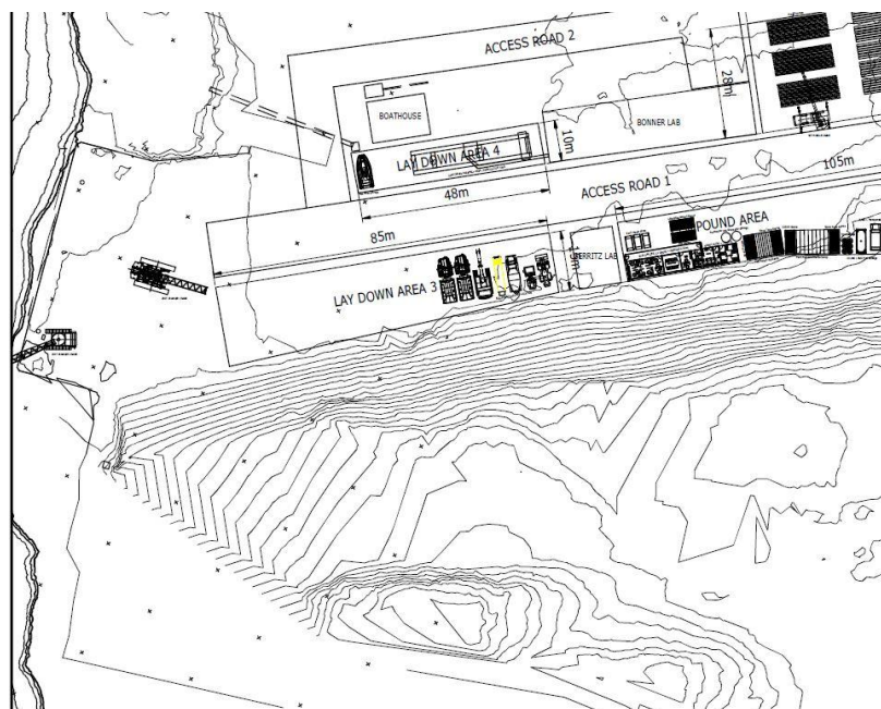
Figure 30 – Laydown area 3 is designated for quarry processing plant.
