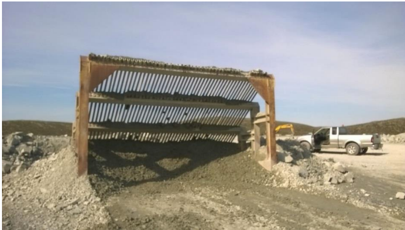
Figure 32 Example of a grizzly screen
