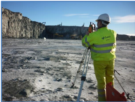
Figure 27 – Undertaking a laser profiling survey of the face
