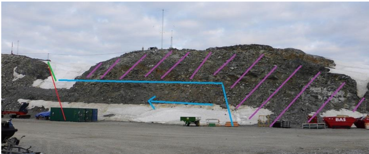
Figure 10 – Quarry stage 3 showing the upper bench worked out and production continuing on the lower bench.
