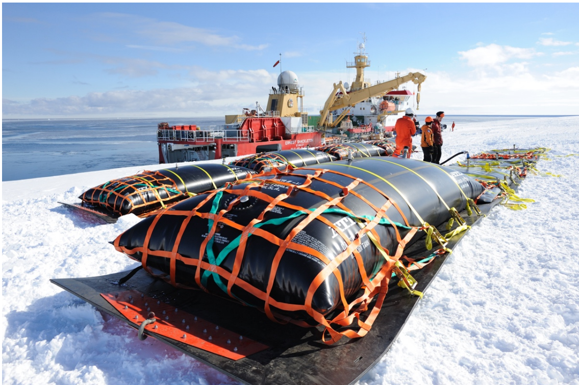
Figure 57. ATL Cargo-Flex™ fuel bladders being filled from the RRS Ernest Shackleton. Source: Wikimedia Commons
