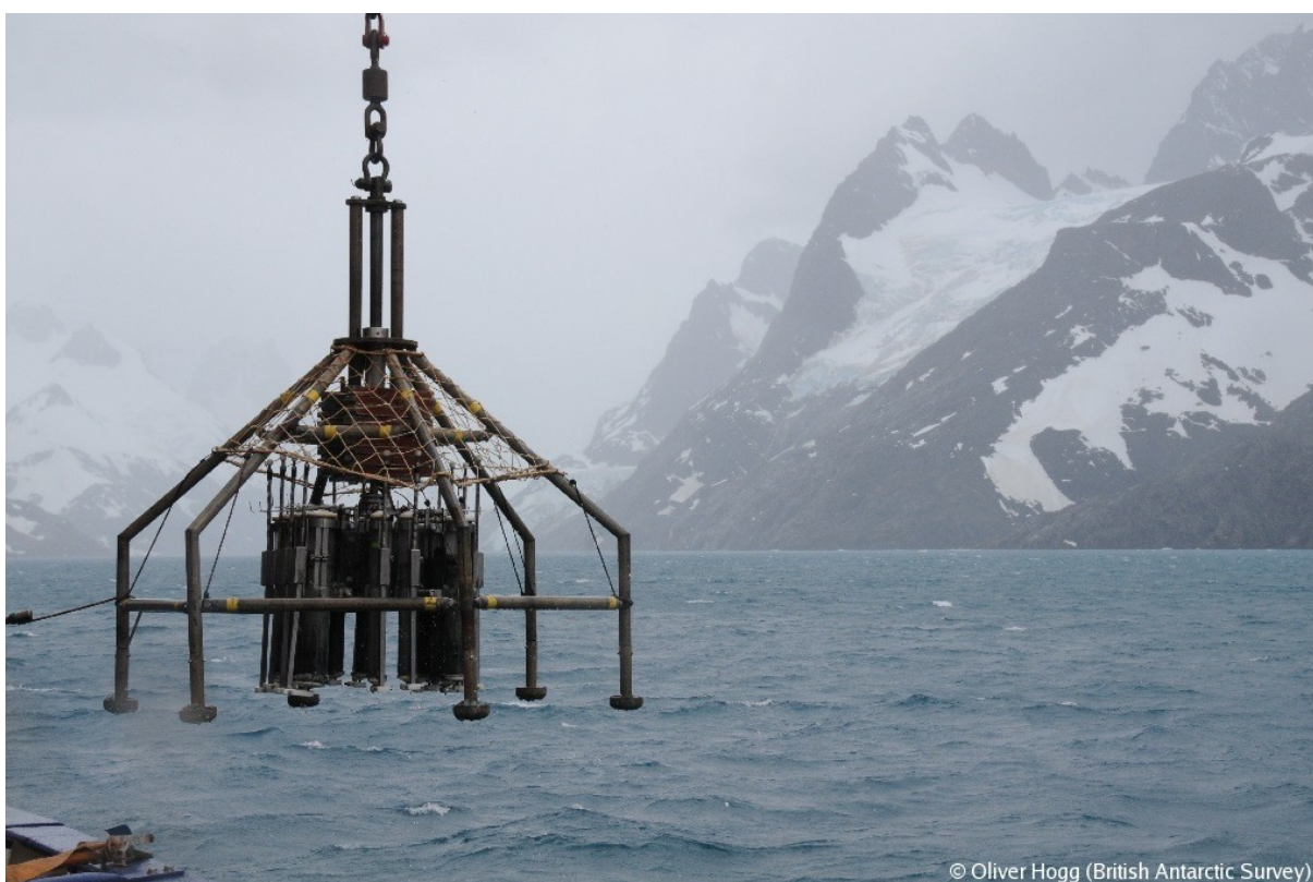
Figure 38. Example of a multi-corer being deployed from RV Meteor around South Georgia in 2017. Photo Oliver Hogg, British Antarctic Survey. Source: http://www.gov.gs/march-17-newsletter/
