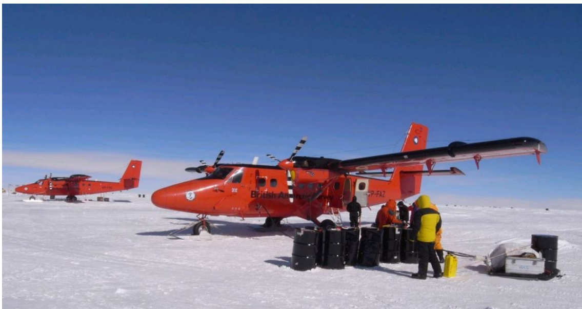
Figure 56. BAS Twin Otter aircraft being loaded with 205 litre fuel drums in the field in Antarctica. Source: www.antarctica.gov.au .
