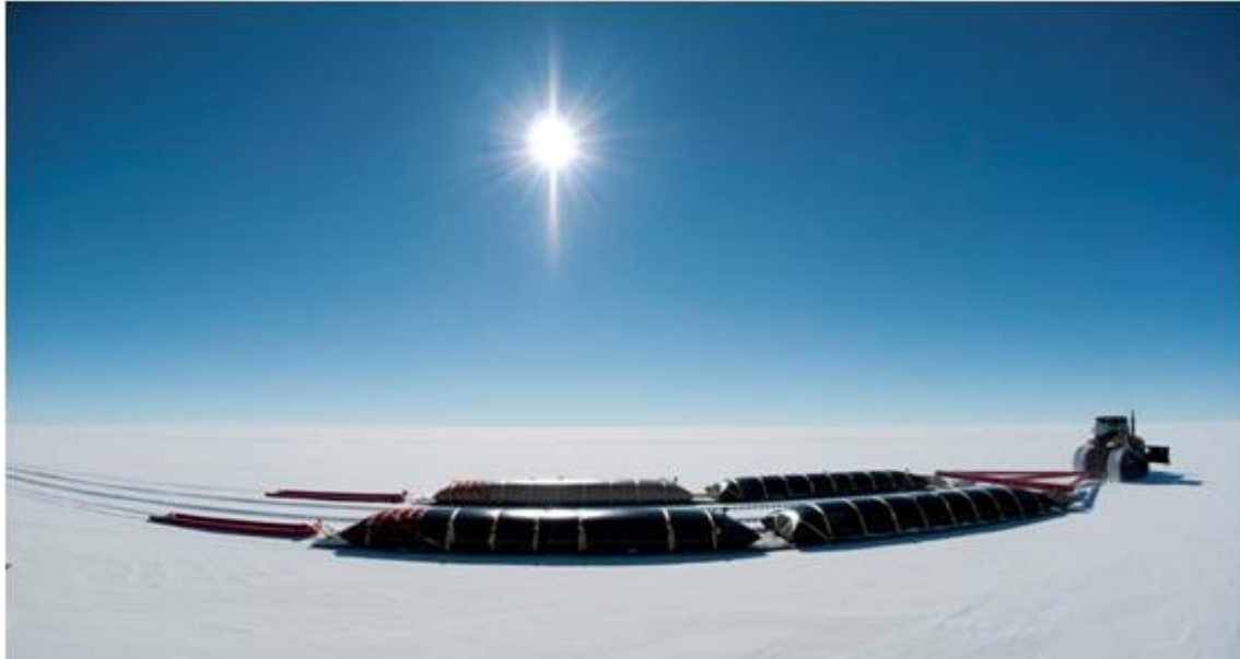
Figure 55. Fuel bladders being towed during the UK iStar research programme. Image: Simon Garrod. Source: www.istar.ac.uk .
