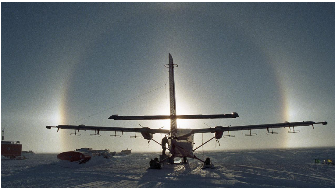
Figure 22. A BAS Twin Otter aircraft equipped with aero-geophysical survey equipment. Image: Sam Witt / British Antarctic Survey. Source: https://www.euronews.com
