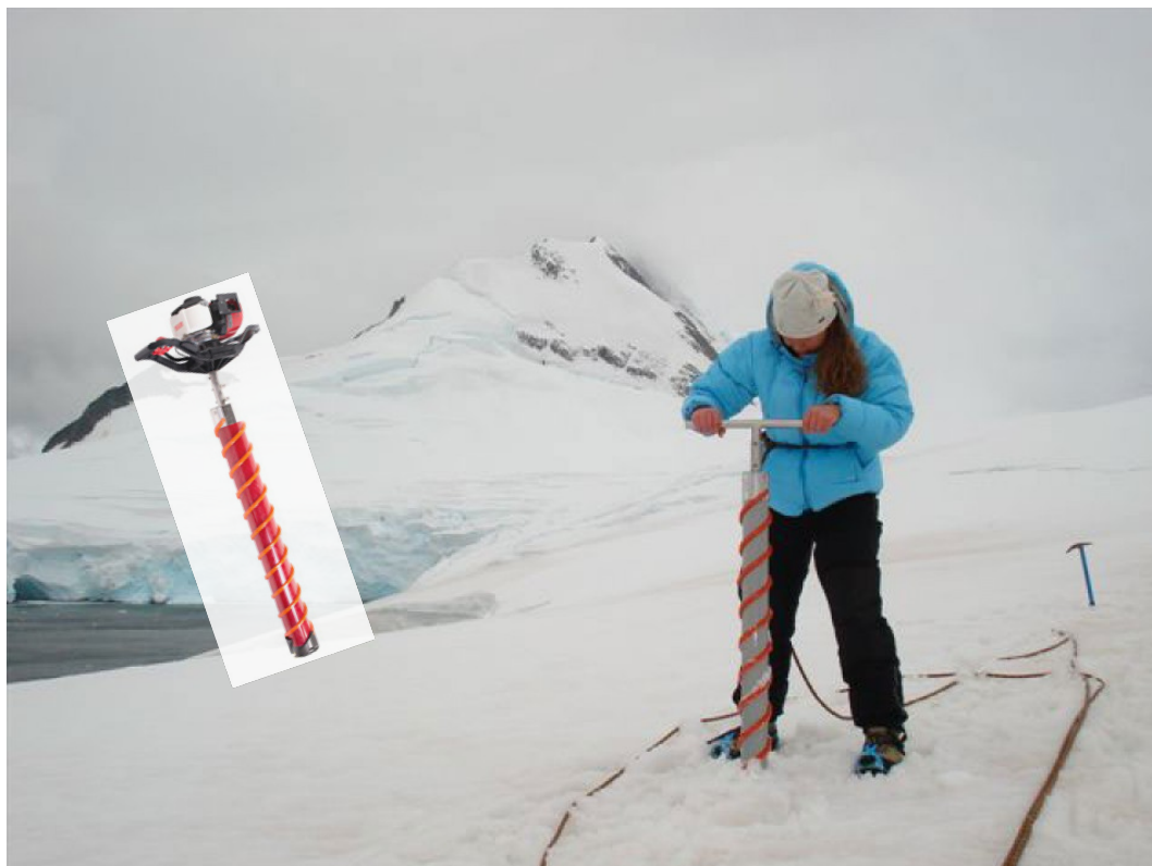
Figure 41. Kovacs ice corer being used in Antarctica. Image shows hand-held and (inset) powered versions. Image: https://kovacsicedrillingequipment.com/photo-gallery/
