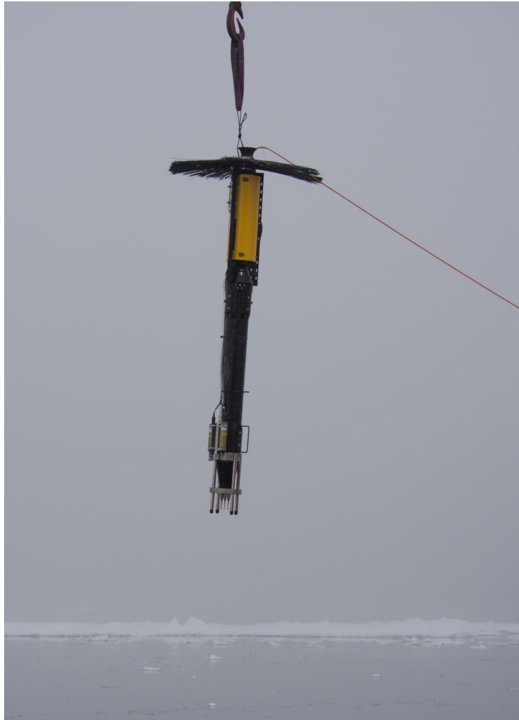
Figure 33. A vertical microstructure profiler being deployed from the RRS James Clark Ross. Image: Povl Abrahamsen, British Antarctic Survey
