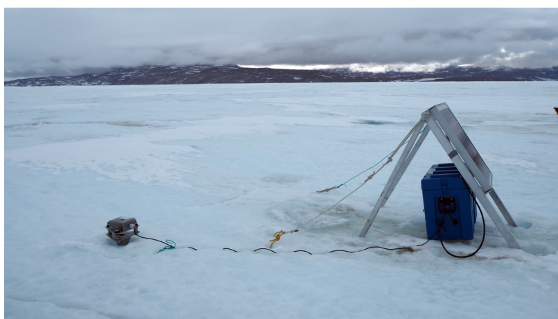
Figure 20. A deployed tiltmeter on the Darwin Glacier, Antarctica in 2016. Image: Dana Floricioiu. Source: https://www.dlr.de
