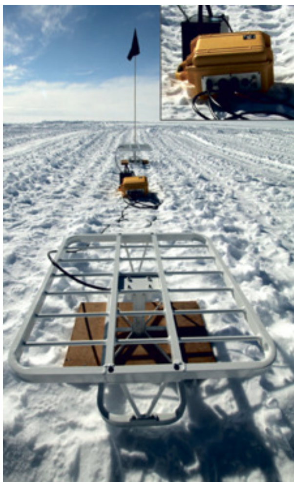
Figure 15. Photograph of an ApRES system deployed on the Ronne Ice Shelf, Antarctica. The ApRES is the yellow case positioned between the two antennas. Source: Nicholls et al., 2015.
