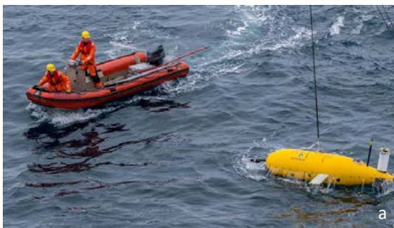
Figure 50. Small rigid-hulled inflatable boats being used to support the recovery of an AUV (a) and to deploy researchers (b). Sources: www.nerc.ac.uk and www.bas.ac.uk .
