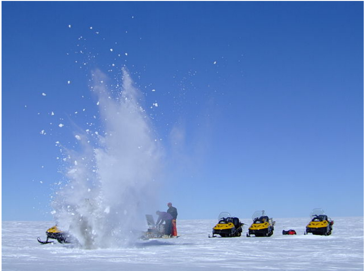
Figure 10. Active seismic measurements being carried out on the Pine Island Glacier, Antarctica. Source: Polargeo, Public Domain
