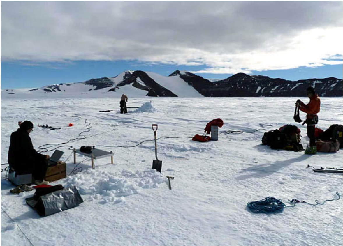
Figure 13. A U.S. field team sets up a magnetotelluric station near the Trans-Antarctic Mountains during the 2010/11 season. Image: Phillip Wannamaker. Source: https://antarcticsun.usap.gov
