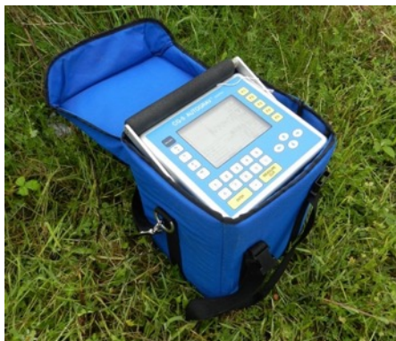
Figure 19. An example of the CG-5 Autograv gravimeter that will be used by the GHOST and TARSAN projects.
