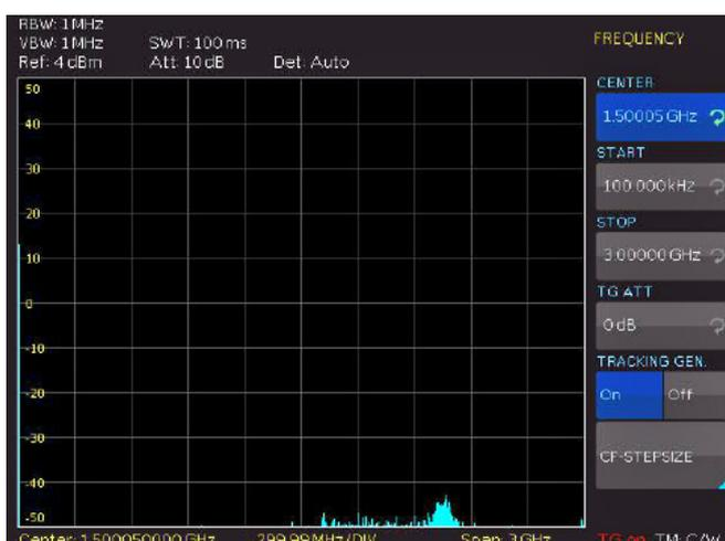
Fig. 6.11: Loosening of the RF cable completely
