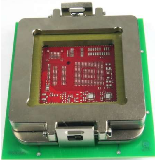
Double Latch Socket w/Center Open
