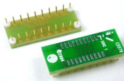
SOIC to DIP converter using blind hole technology
