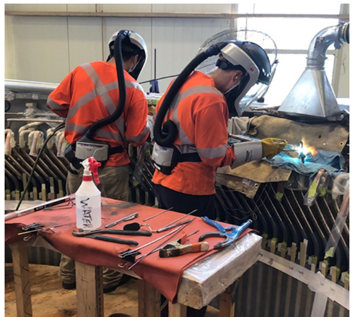
Winders brazing copper coil connections. Oxygen/acetylene torches were used with extreme caution.
