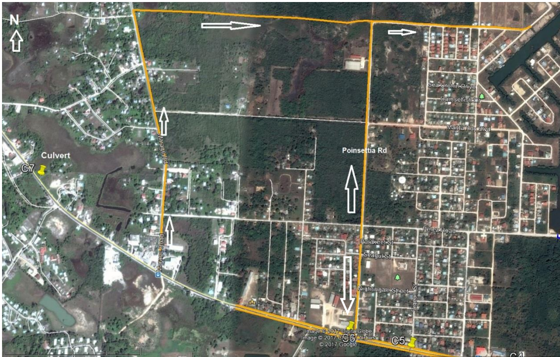
Figure 6.15: Improved drainage along Poinsettia Street and Marage Road, Ladyville, eastwards then southward to the Vista del Mar Canal.
