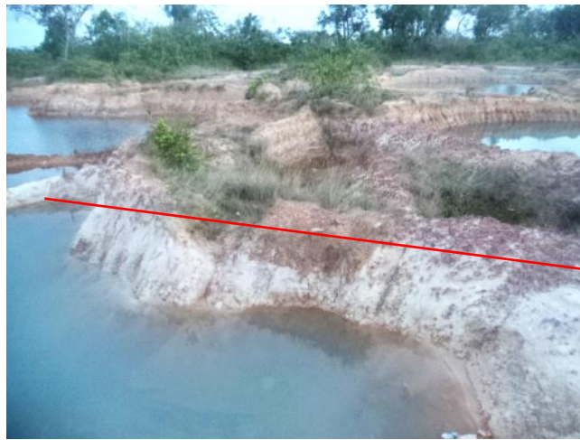
Figure 6.10: Typical clay, clay and chert fill extraction site, showing isolated and sterilized materials due to water invasion.
