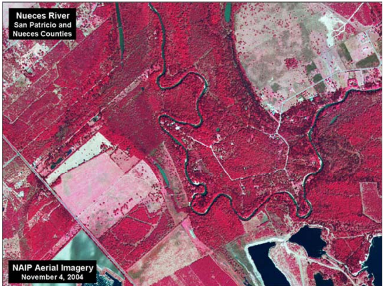
Figure 4. Example of one-meter color infrared ADS40 imagery collected in 2004 for the USDA National Agricultural Imagery Program. Note the contrast in vegetation appearance near the banks of the Nueces River with areas in the surrounding agricultural fields and scrubland. The imagery is not shown at full resolution.
