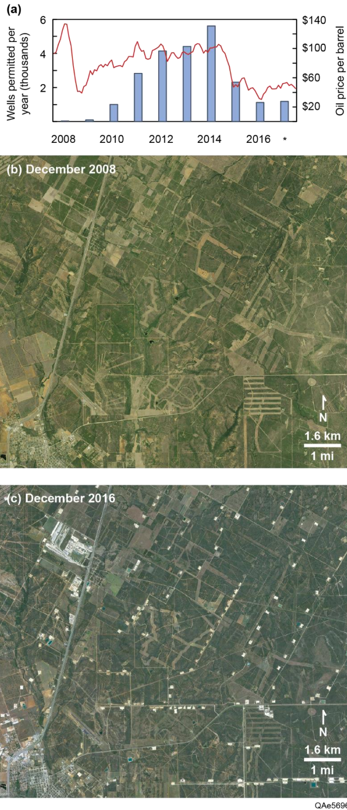
Figure 11.1. Eagle Ford drilling and oil price history Price history (a) and resulting landscape alteration from December 2008 (b) through December 2016 (c) for a representative portion of the play northeast of Cotulla, TX (southwest corner of
