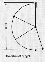
180-degree 3-Panel Sweep Pen with a 10' Straight lead-in Panel.
