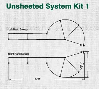
180-degree Sweep with 10' Straight lead-in Panel with 20' of Adjustable Straight Crowd Alley. Includes Drop Down No Back.
