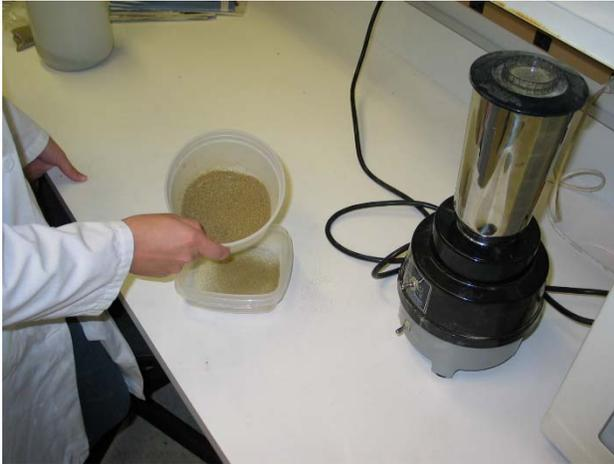
**Figure 1.3.2.1.** Preparing food. Use a general laboratory grinder (pictured here), a grinding mill or a household coffee grinder, or mortar and pestle. To ensure food is small enough for the earliest stages, use a sieve with holes no larger than 250 microns in size.
