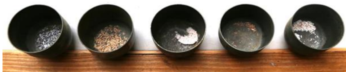
Figure 8: Ash residue after the muffle furnace, shows varying ash colors and textures between different species, which could affect burning processes and should be further explored in future studies.
