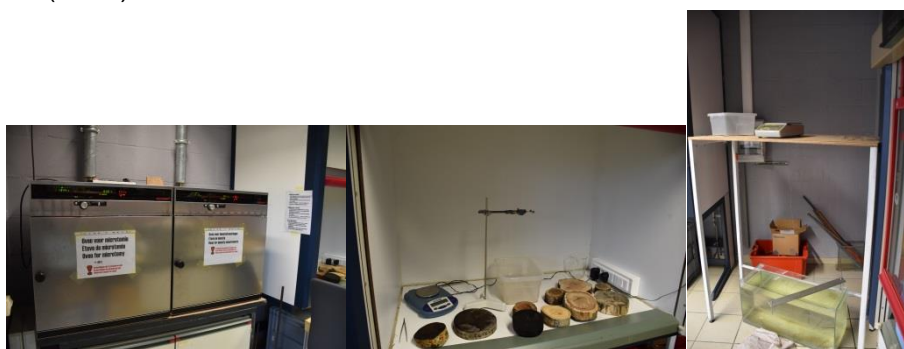
Figure 6: Setup for the oven-dry wood density measurements with the water displacement method at the Royal Museum for Central Africa (Service of Wood Biology). Left: ovens to oven-dry the wood samples, Middle: scale and water displacement for small samples, Right: scale and water displacement for large samples.
