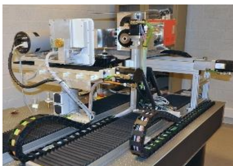
Figure 4: Setup of X-ray Computer Tomography toolchain at Woodlab, Ghent University
