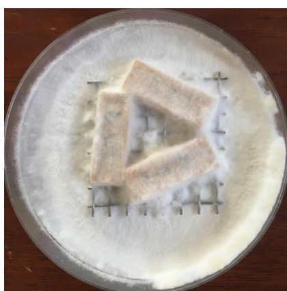
Figure 3: Beech mini-blocks within a petri dish overgrown with Trametes versicolor . The mini-blocks are placed upon a metal grid, to avoid direct contact with the agar. From Deklerck et al. (2019, under review).
