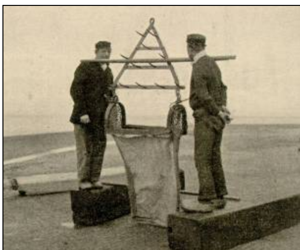
Figure 2: The "drague à anses", here equipped with the frontal rake (source: Gilson, 1900)
