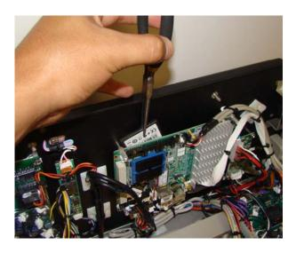
7.1.4 To re-install a card place it in the slot, then press it in until you feel it latch into place. A small screwdriver or pen may be required to fully insert.
