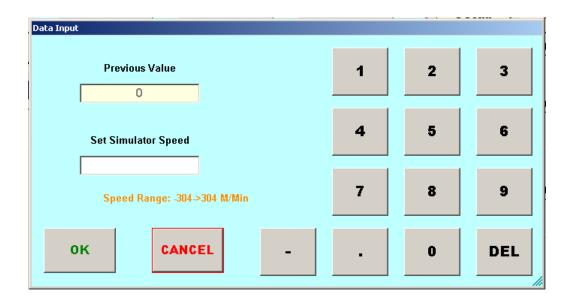
The simulator is handy for testing purposes only. Simulated depth is produced by software and if the panel is set to corrected out mode (refer to 3.5.14) the panel will produce simulated corrected output pulses.
