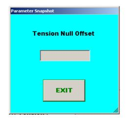
This value is derived from the tension zero function in the tension calibrate menu (3.2.1).
