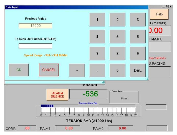
This provides a means to re-scale the output signal. The default is 12,500 lbs = 10 volts out.
