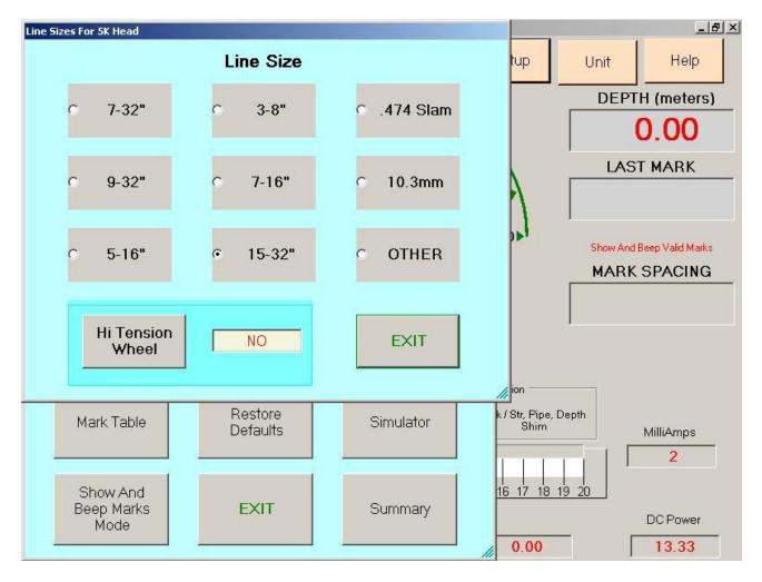
The selection of the 9 built-in line sizes and the deep grooved (Hi-Tension) wheel is specifically for use with the Benchmark 5K Head.
