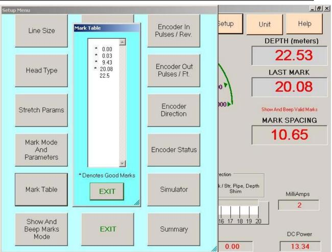
This table allows the viewing of all the Marks found while logging. This can help in differentiating between good marks and false marks.
