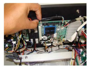
7.1.2 Using a pen or small screwdriver press the reject tab. The card will then pop out of the holder.
