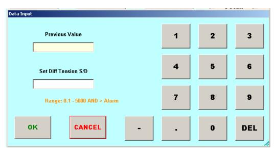
The Set Differential Tension S/D entry screen will appear. The range is 0.1-5000 AND > Alarm.
