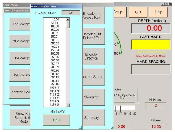
This is the table of the location of the magnetic marks on the cable based on: line size, line weight, line volume, line stretch coefficient, tool weight, and mud weight. Note the text box labeled 'FIRST MARK OFFSET'. For Example: If the value is 10.00 Meters, then all numbers in the table reflect the theoretical mark...eg... 50M plus the first mark...eg... 10M Equals 60 Meters for the actual location of the mark.
