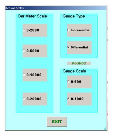
The Tension Scale Screen allows the changing of both Bar Meter Scale near the bottom and the Needle Gauge Scale at the center of the screen. It also allows the Gauge Scale to be used either in a Differential or Incremental scale.
