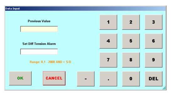
The set differential tension alarm screen will appear. The range is 0.1 - 2000 AND < S/D.
