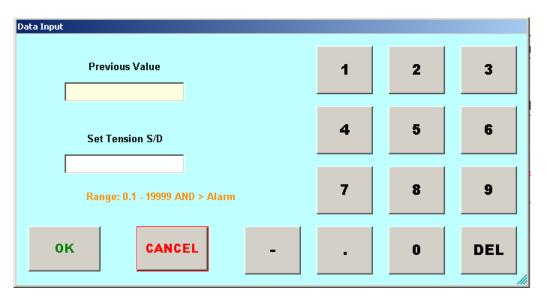
The set tension shutdown screen will appear. The range is 0.1-19999 and > Alarm.
