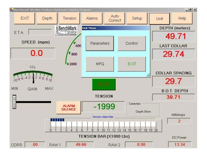
**UNIT:** For this Revision the unit menu is inoperable. Future Features will include the ability to choose Hydraulic Winch Control, Manufacturer, And Parameters for can communications control.
