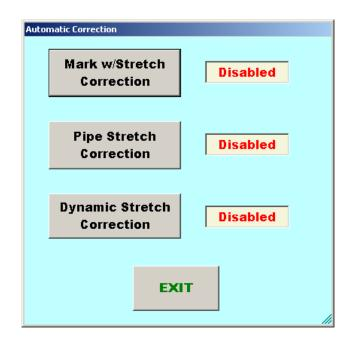
This menu allows changes to be made to the stretch correction mode as required by the wireline, drilling mud and logging tools that are being used on the job.
