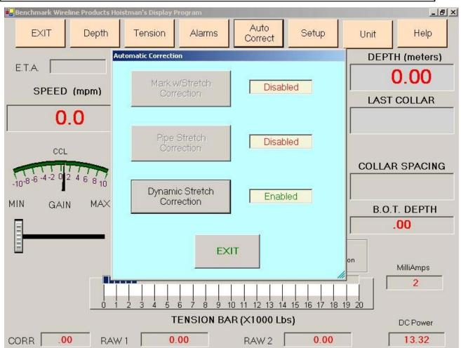
NOTE: When Dynamic Stretch Correction is enabled, Mark with Stretch Correction and Pipe Stretch Correction cannot be enabled.
