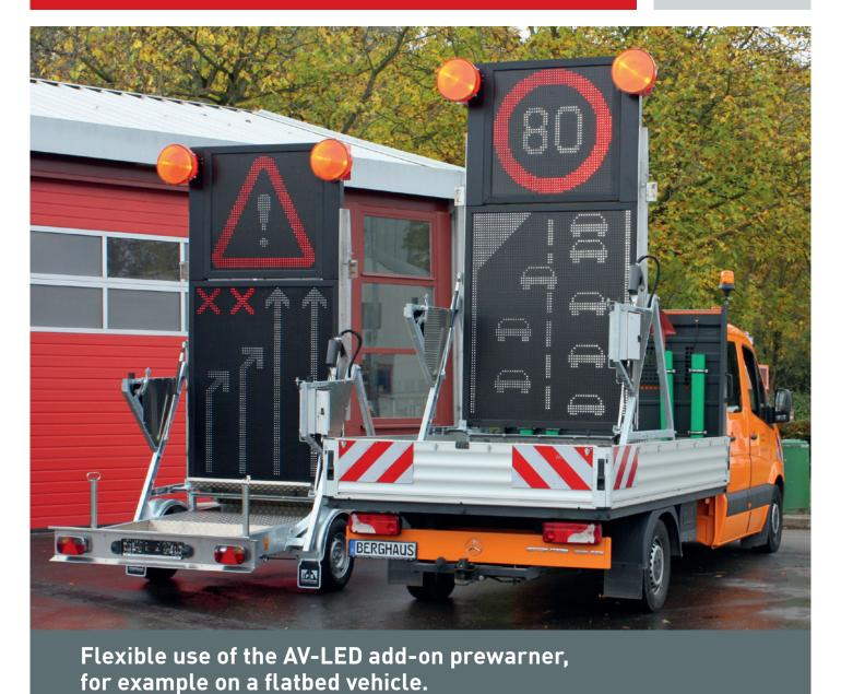
Our proven MV-LED mobile prewarner is also available in a version without chassis. The AV-LED add-on prewarner can be placed quickly and easily on the loading
