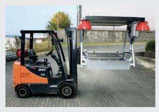
When the need arises, simply use a forklift truck to place on the loading area of the required transport vehicle: secured at the fastening eyes, the AV-LED is immediately ready for professional traffic safety use with practically any flatbed vehicle.
