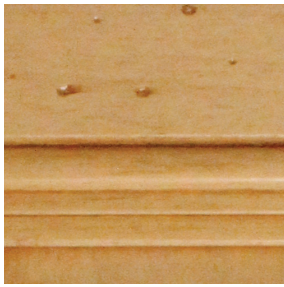
#1 - NICKS & DENTS Small, random nicks, dents and dings in the wood substrate.
