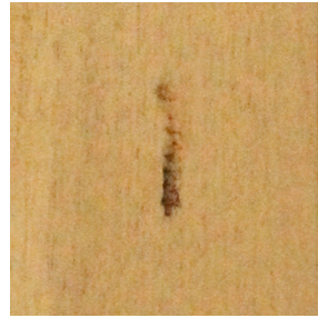
#3 - SCREWMARKS Random screw impressions on the wood showing thread marks.
