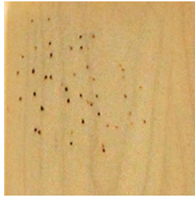
#2 - BIRD PECKING Small randomly grouped holes, simulation bird pecking.
