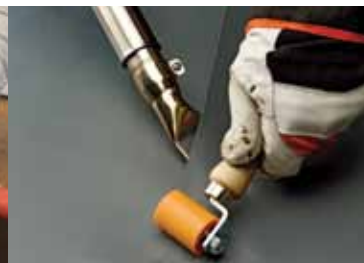
DW 2000 hot-air tool & rollers
