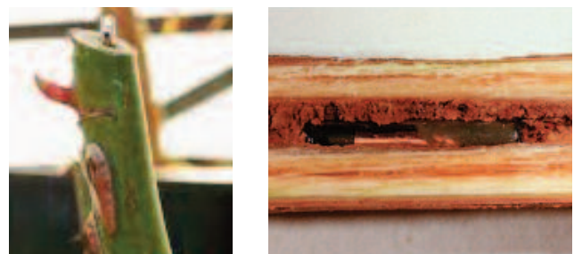
RFID chip implanted in a rose (left) and grapevine (right) and used in trials for certifying stock, monitoring pests and mapping. (Images: Associazione Toscana Costitutori Viticoli)
