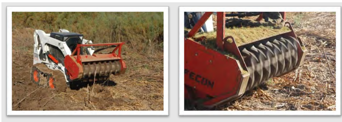
Figure 9-2. A Bobcat with a brush hog mower attachment removing noxious weeds. Photo courtesy of Fred Phillips Consulting, LLC.
