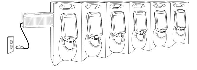
Figure 50 Maximum Number of Charge Cradles per Power Supply with "Y" Power Cable
