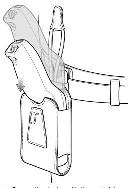
4. Secure the device with the restraining strap and place over the device and hook to secure in place.
