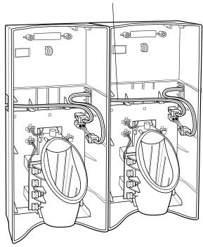
5. Use plugs to cover un-used cable outlets.
