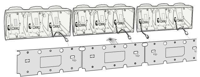
**6.** Secure the back cover of each cradle using six T10 Torx screws (supplied). Torque screws to 6 Kgf-cm (5.2 in-lb).
