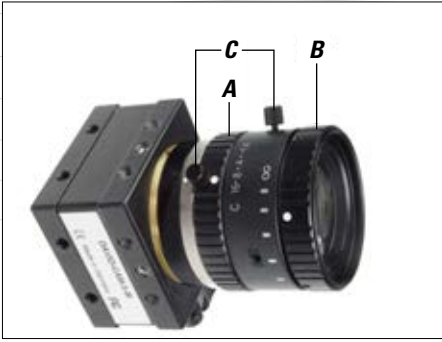
Figure 4.2: Adjusting rings (A) aperture and (B) focus, (C) fixing screws
