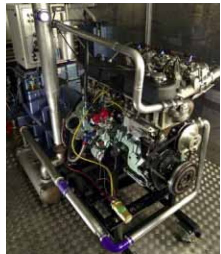
Healey 3000 engine gets put through its paces on our Dynamometer.
