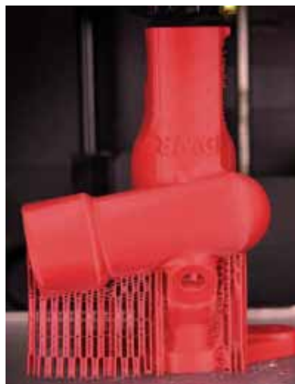
100S tacho tower 3-D printing of prototype
