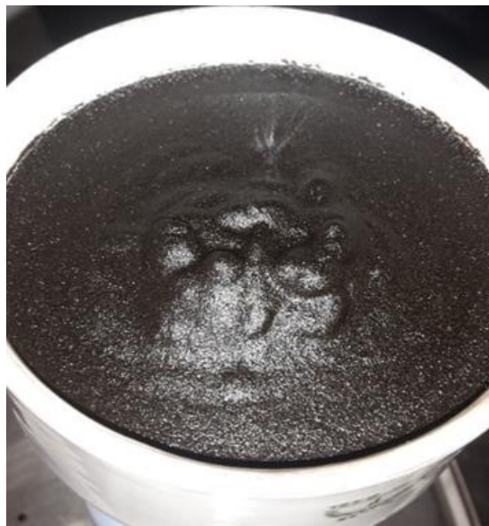
Figure 49: HTL crude produced from black liquor (Source: VTT)
