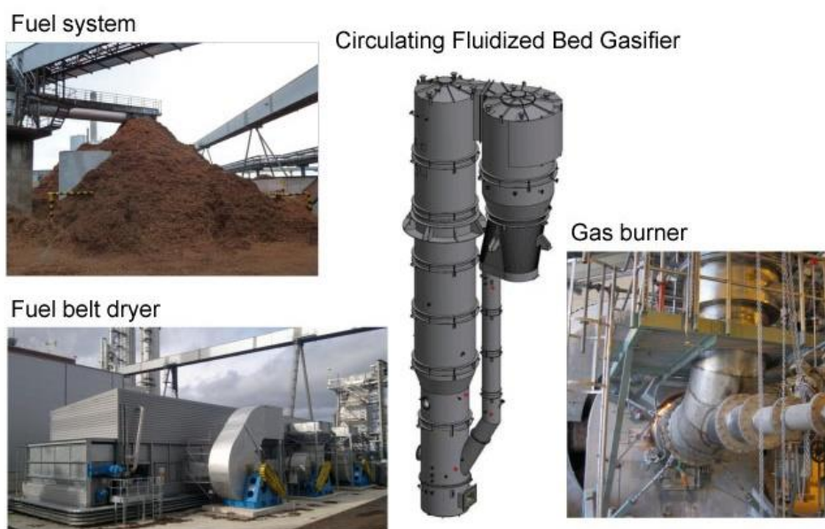
Figure 51: Components of a gasification plant (Know pulp, 2019)
