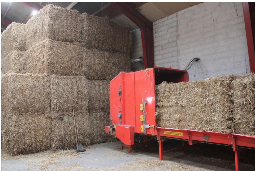
Figure 11: Straw bale feeding system for a district heating grid in Denmark (Source: D.Rutz)
