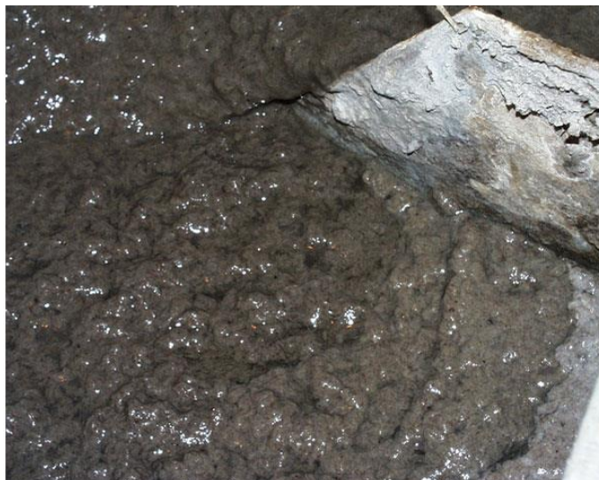
Figure 47: Sludge from pulp mill wastewater treatment (KnowPulp, 2019)
