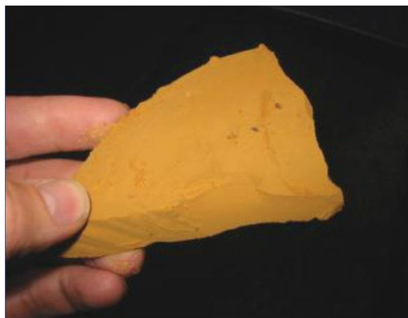
Figure 48: Lignin separated from the Kraft process (KnowPulp, 2019)
