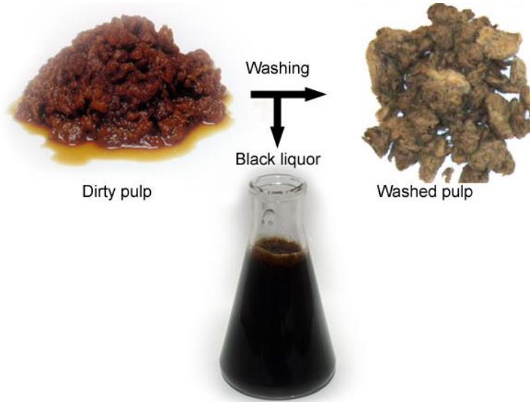
Figure 38: Washing of dirty pulp produces black liquor and washed pulp (KnowPulp, 2019)
