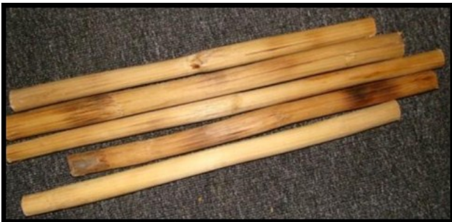
Fig. 2- Oil Cured Rattan after Six Weeks Exposure to Termites.
