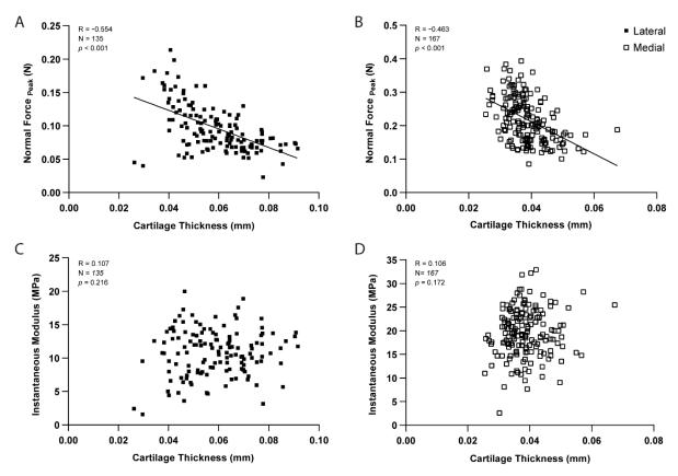
**Figure 3.** Correlation graphs per testing site for the lateral (n = 135 positions) and medial (n = 167) condyles, showing cartilage thickness (needle probing) is significantly correlated to peak indentation force at 20 um (A-B), but not to instantaneous modulus values as determined by Hayes *et al.* (1972) elastic model at 20% strain. p-values reported.
