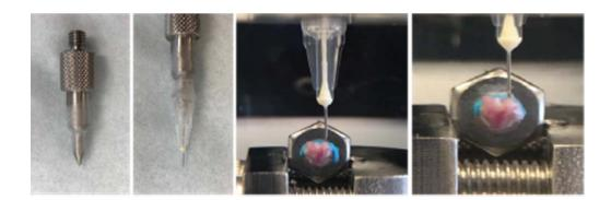
**Figure S2.** Setup for needle probing thickness measurement, using a 30G x 1.4" hypodermic needle (TSK Laboratory, Japan) adapted to the 1 mm spherical indenter (*Biomomentum Inc.*, Laval, QC).
