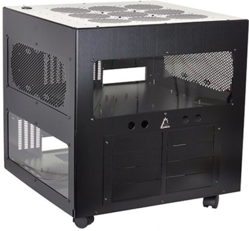
Figure S8. Phobya WaCoolT Cube 2 Watercase was modified to serve as external case for the OptoGenBox. This figure was reproduced with permission from Performance PCs.
