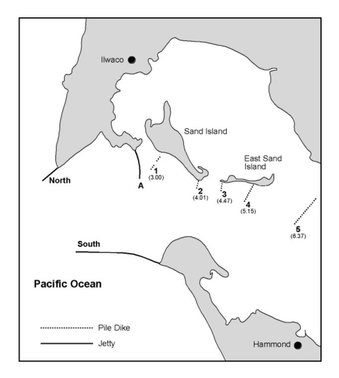
**Figure 1.** The jetties and pile dikes at the mouth of the Columbia River. The river mile for each pile dike is shown in parentheses under the dike number.
