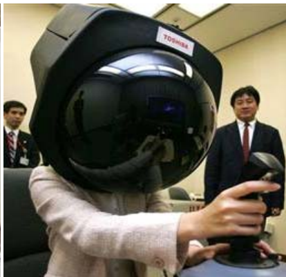
Figure 5: Trimersion head-mounted display and instrumented weapon for gamers (left), Toshiba "Bubble Helmet", originally demonstrated in 2006 with Microsoft's Flight Simulator (middle) and Novint's $189.00 (August 2008) Falcon haptic (force/touch) feedback system (right).
