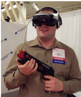
Figure 5: Trimersion head-mounted display and instrumented weapon for gamers (left), Toshiba "Bubble Helmet", originally demonstrated in 2006 with Microsoft's Flight Simulator (middle) and Novint's $189.00 (August 2008) Falcon haptic (force/touch) feedback system (right).
