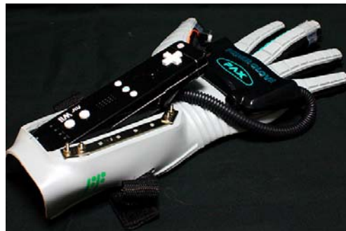
Figure 52: Mattel Power Glove , modified using a Nintendo Wiimote .
