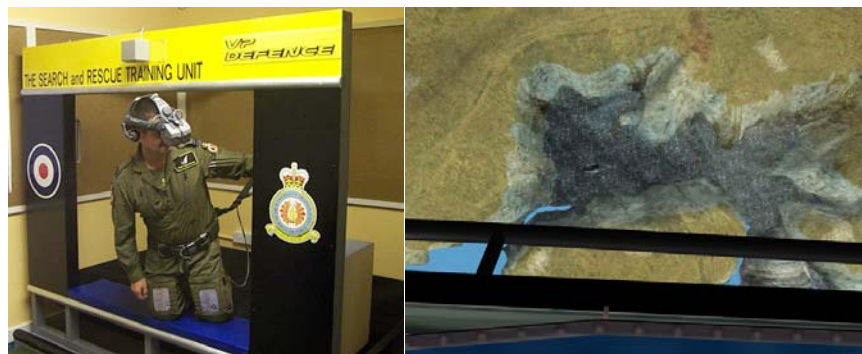
Figure 42: Helicopter voice marshalling VR solution – simulator station (left); view from virtual cabin (right).
