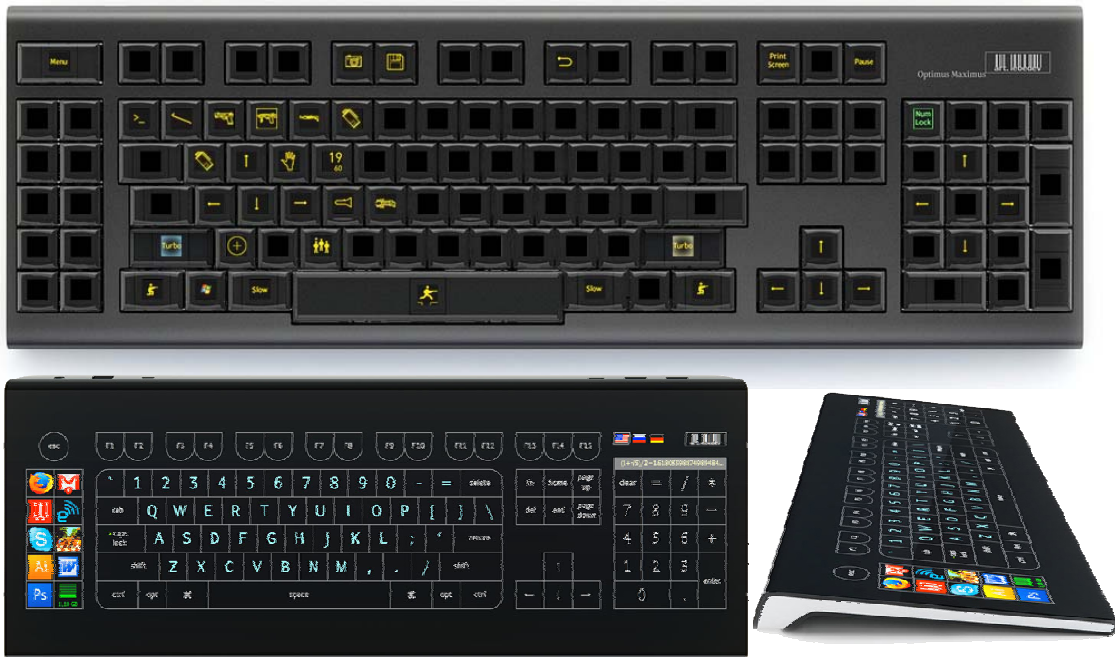
Figure 51: Art.Lebedev Studio's Optimus Maximus (Upper) and Tactus (Lower) programmable keyboards (note that the keys on the Maximus have been programmed to support the game Half-Life ). Source: www.artlebedev.com
