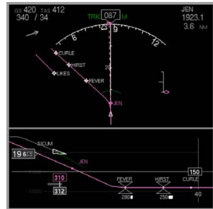
Figure 36: Example of an avionics coplanar display (map Display on top, VSD Below).
