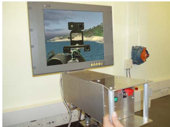
Figure 10: HFI DTC desktop Minigun trainer. Source: Author’s Image Archive
