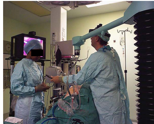
Figure 37: Head-controlled endoscopic camera robot affects “keyhole” surgeon’s posture and medical instrument working envelope. Source: Author’s Image Archive
