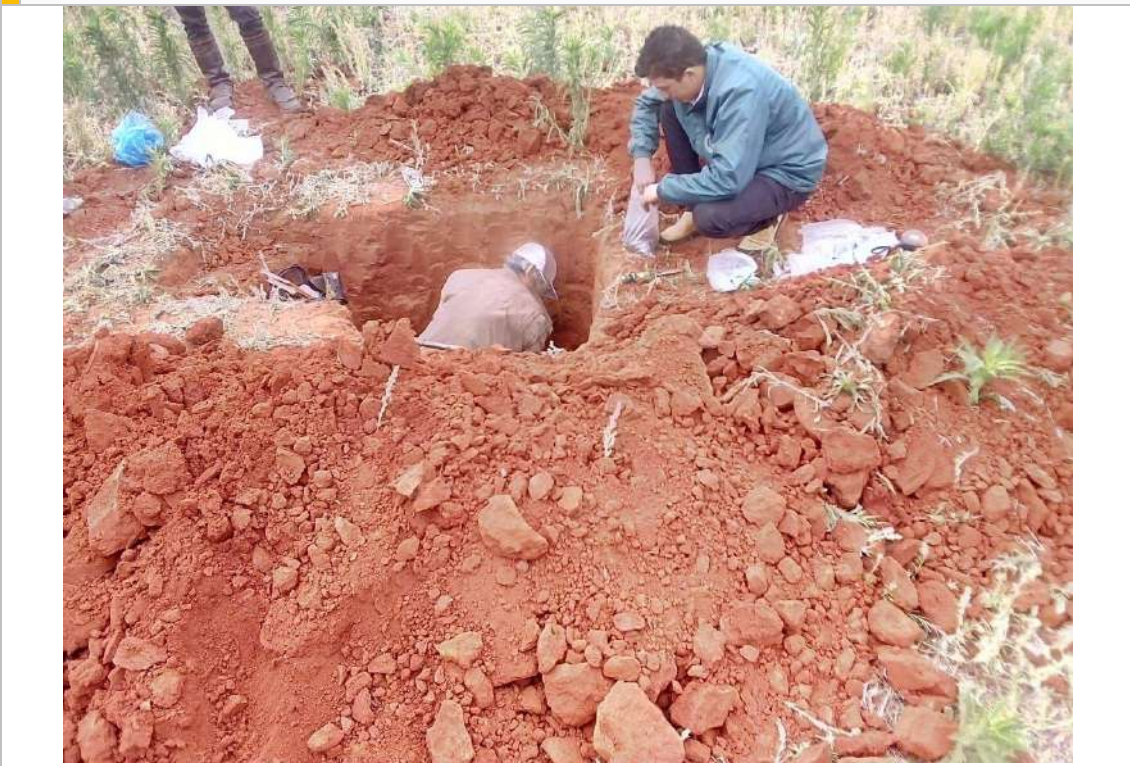
Trial pit east of the property
