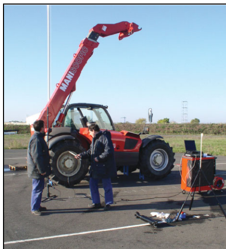
Fig. 8 Sound intensity measurements are made using Sound Intensity Probe Type 3599, PULSE and Noise Source Identification Type 7752.
