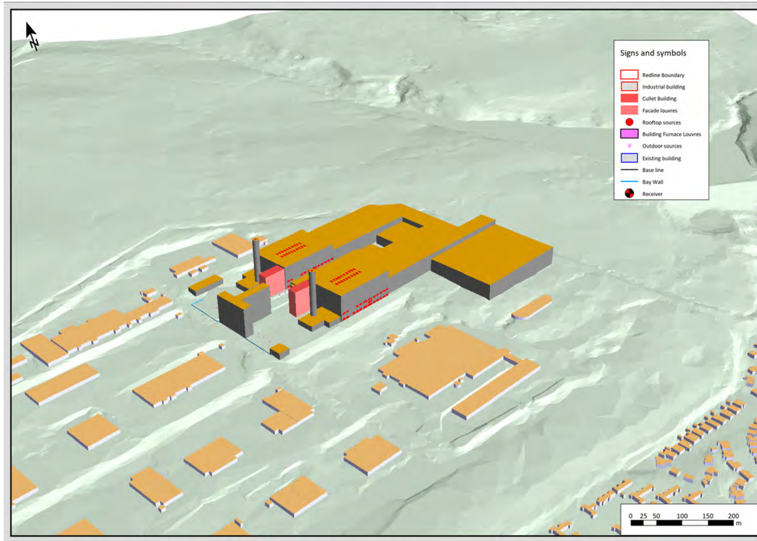
Figure F4.5: Perspective view of the proposed development and modelled noise sources
