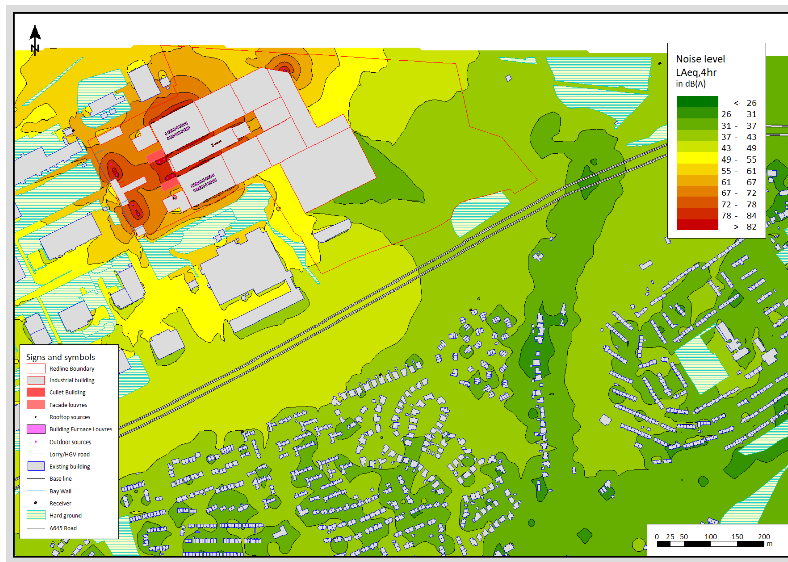
Figure F4.7: Grid noise map of the proposed development during normal evening operation - only proposed facility noise sources
