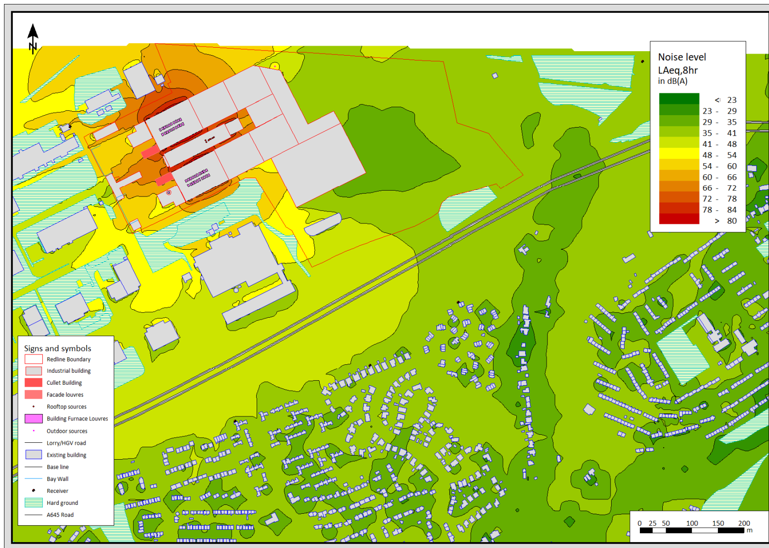
Figure F4.8: Grid noise map of the proposed development during normal evening operation - only proposed facility noise sources
