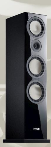
The Canton Chrono series offers advanced technology for improved transparency and control. Titanium double cone woofers feature an advanced wave-surround allowing greater excursion and higher sound output with lower distortion. The high-density cabinet reduces unwanted resonance and features a high-gloss lacquer front baffle with elegant aluminum trim rings surrounding the woofers. The rest of the cabinet is finished in a black or white matt wrap. The enclosures are rear-ported.
