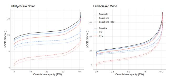
Figure 6. Utility-scale solar and wind supply curves for alternative policy scenarios for 2030. These curves are a transposition of the maps in Figure 5.
