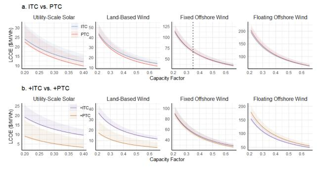
Figure 3. Levelized cost of electricity (LCOE) for each technology with respect to capacity factor. The impact of capacity factors is evaluated for the *base* (a) and *bonus* (b) tax credit rates. The LCOE for 2030 is depicted by solid lines, while the shaded regions represent the potential range of LCOE values from 2023 to 2050. The vertical dotted lines represent capacity factors, where the minimum LCOE shift occurs between policy scenarios.
