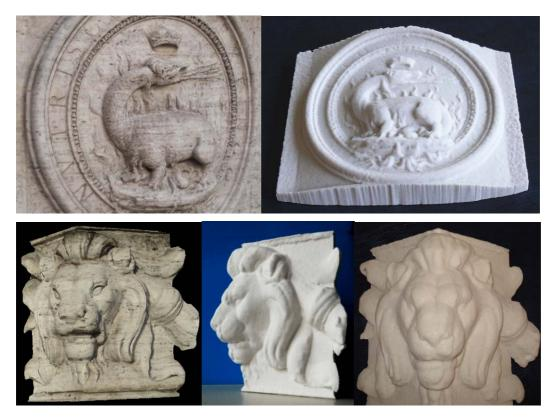
**Fig. 5.** Textured digital models and replicas printed with resinated chalk. The undulate edges are due to an automated elaboration (exception made for the scale of the model, the selection of the printable area, and the thickening of the reconstructed surface). To obtain sharp edges a manual editing is needed
