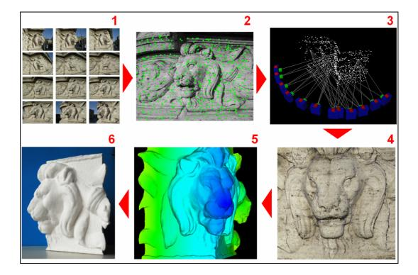
**Fig. 2.** The pipeline of the proposed procedure for 3D modeling and physical replica creation. It is interesting to notice that the image correspondences in 2 and 4 are automatically detected
