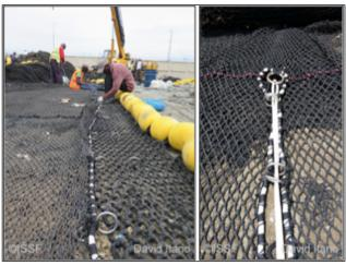
**Figure 9.1**. Construction of the top portion of the release panel (left) and detail of rings at the bottom corner (right).
