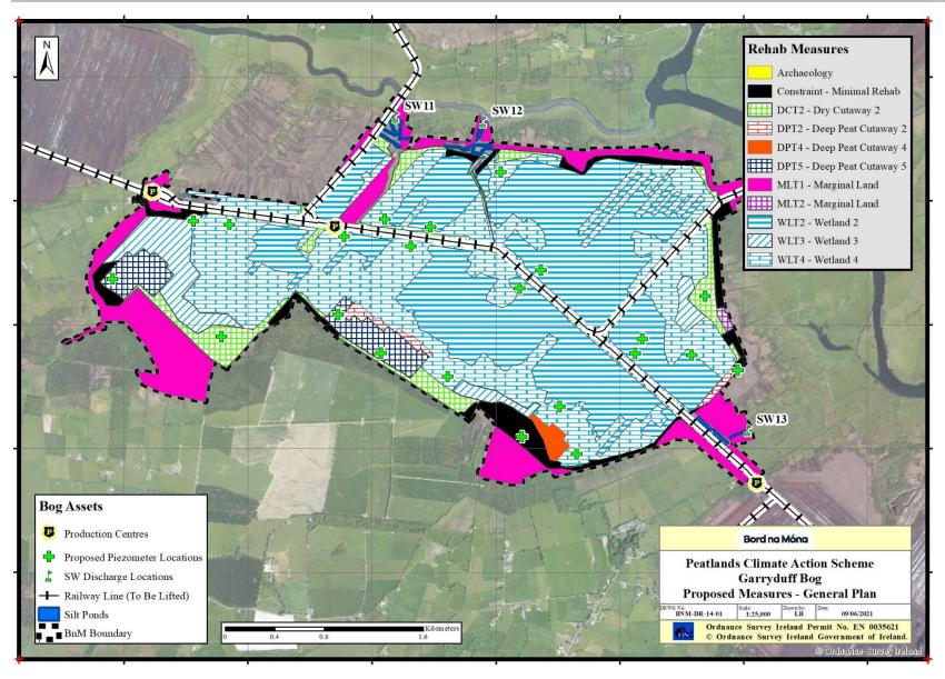
Figure 8.5. Indicative Enhanced Rehabilitation Plan for Garryduff Bog. *Note that the types of rehab and areas of rehab may change in response to stakeholder consultation and* refinement of the enhanced rehabilitation measures.
