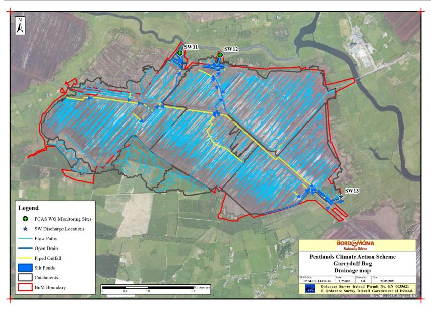
Figure 3.5a. Map of Garryduff Bog showing water management features and water quality monitoring points.
