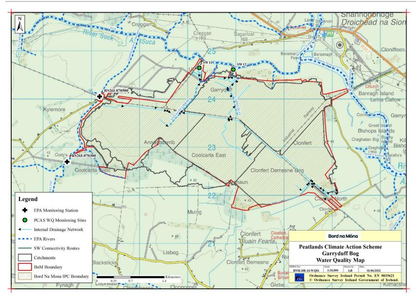
Figure 3.5. Map of Garryduff Bog showing water management features and water quality monitoring points.
