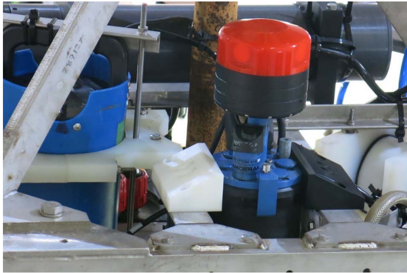
Figure 13 - The Seaguard in the sensor frame on the day of deployment (18/04/17) with the cap still on the optode to keep it moist (removed before deployment). The clamps on top were secured to keep the Seaguard in place.
