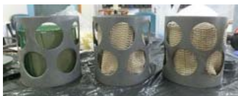
Figure 56. Wood substrate baskets prepared for Bathysnap deployment.
