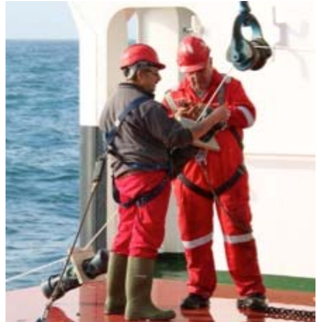
Figure 54. LO 3 CAted settlement frames and larval traps being recovered from PAP#3 mooring line 45m below sediment trap 4732m.
