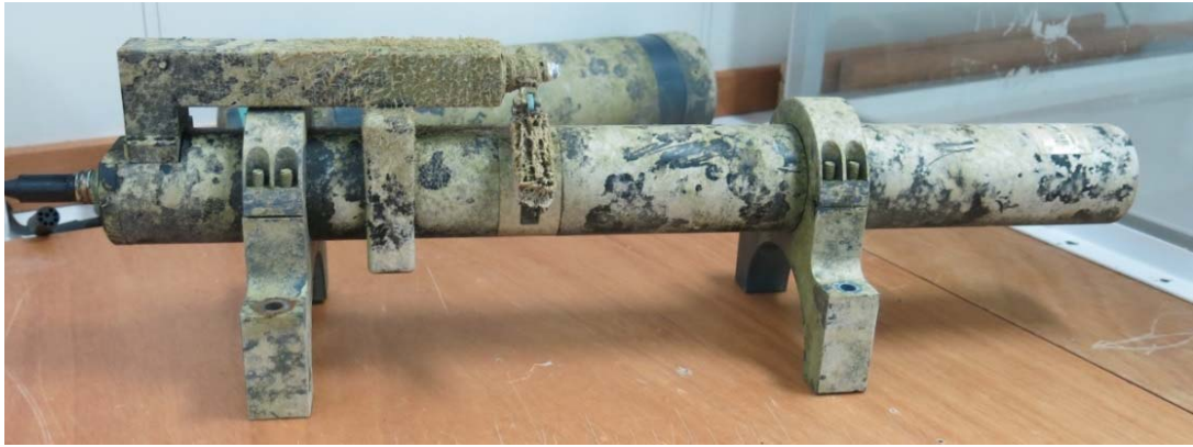
Figure 28: Satlantic SUNA Nitrate sensor recovered from the sensor frame one year after deployment. Biofouling likely biased the nitrate concentration data.
