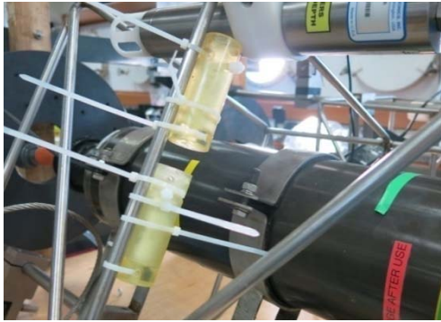
Figure 37: Star ODDIs attached to the frame of the SAP unit for a post-recovery calibration test
