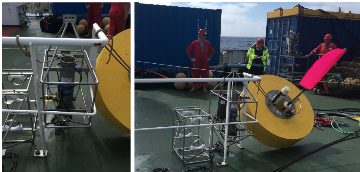
Figure 19: left: RESPIRE trap waiting for deployment; right: surface buoy with light, flag and GPS tracker.
