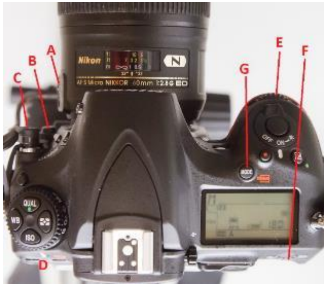
Nikon D810 showing location of major controls used in setting up camera for krill photography
