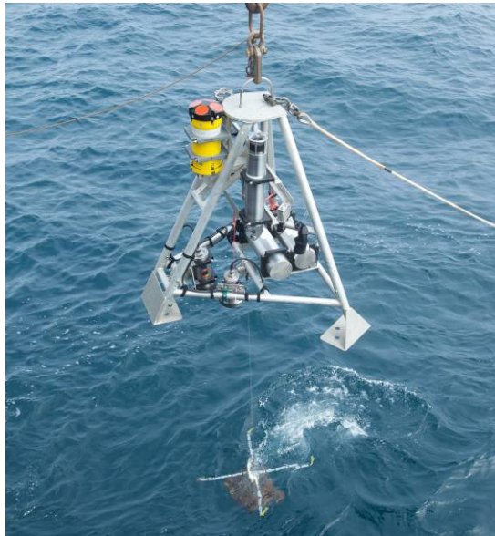
Fig 1: Photographic and Acoustic Lander (PAL) being deployed. Photo courtesy of David Shale.
