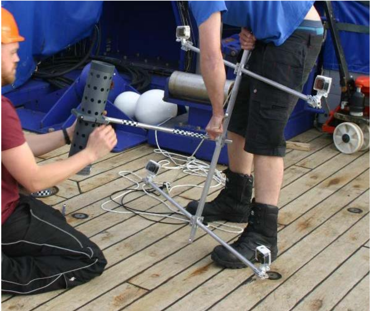
Figure 13.1. – Four Eyes camera frame being set up.
