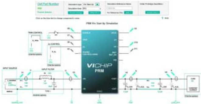
Figure 4: The versatile PowerBench Simulator allows you to test modular power components over seven simulation types: VIN start-up, EN start-up, steady state, EN shutdown, VIN step, load step, and thermal.
