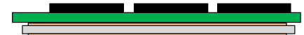
Figure 1d: Side-View of Non - Isolated PPCB Inverter with Three \mu MaxPak HB and DBC Isolator of Bottom-Side
