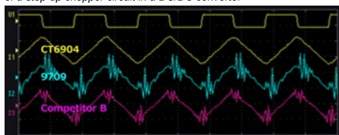
Figure 21: Example of measuring the switching waveforms of a reactor (100kHz switching frequency)
