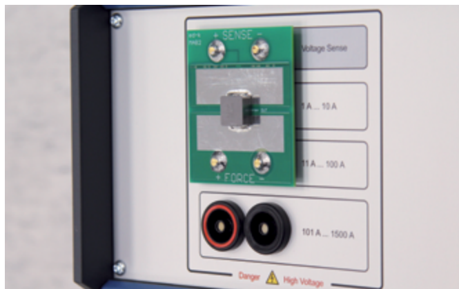
Figure 8: Test adapter MAB1/2/3 for the Power Choke Tester DPG10 series
